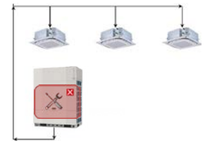
Refrigerant stored in IDU
