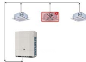
Refrigerant stored in ODU
