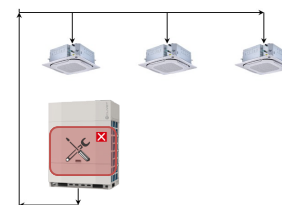
Refrigerant stored in IDU
