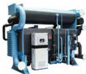
SS/HS Series Capacity: from 350 to 12.300 kW Heat source: Steam (SS)/Superheated water (HS) Steam pressure: 0-3,5 bar g Superheated water temperature: 120-150°C COP: 0,7-0,75
