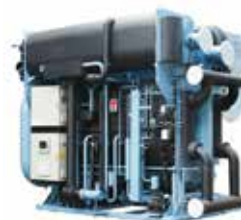
EJ Multi Energy Series Capacity: from 350 to 12.300 kW Heat source: Exhaust gases+Hot water Exhaust gases temperature: 250-600°C Hot water temperature: 80-120°C COP: 1-1,1
