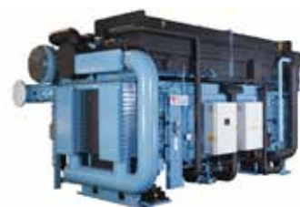
3G Series Capacity: from 176 to 5.300 kW Heat source: Superheated water Superheated water temperature: 180-240°C COP: 1,6-1,9
