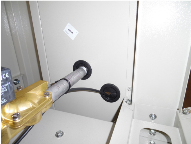
m) Pass the female connector through the lateral panel and connect it with the male one from motorized drain valve
