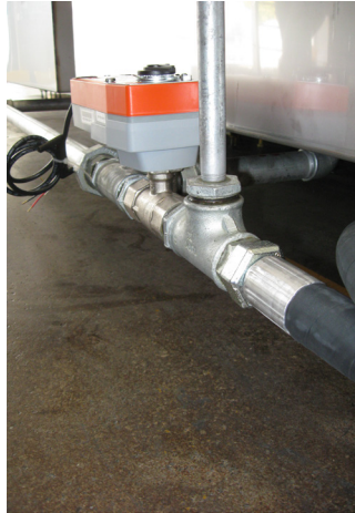
m) Pass the female connector through the lateral panel and connect it with the male one from motorized drain valve
