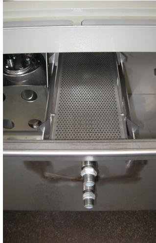
e) Mount the fill-in circuit (part 2) fixing the 3 pieces joint
