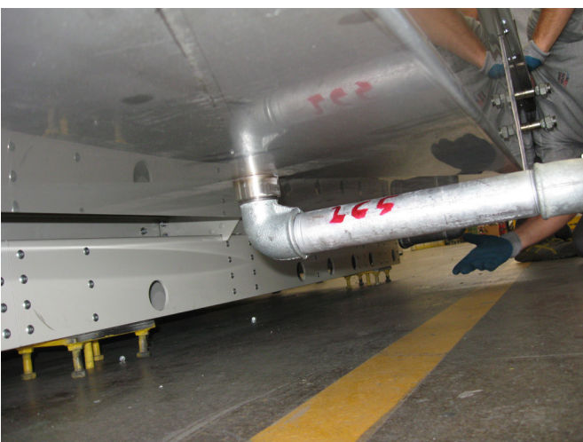
g) Mount a part of drain circuit secondary tank (without bleed-off tank)
